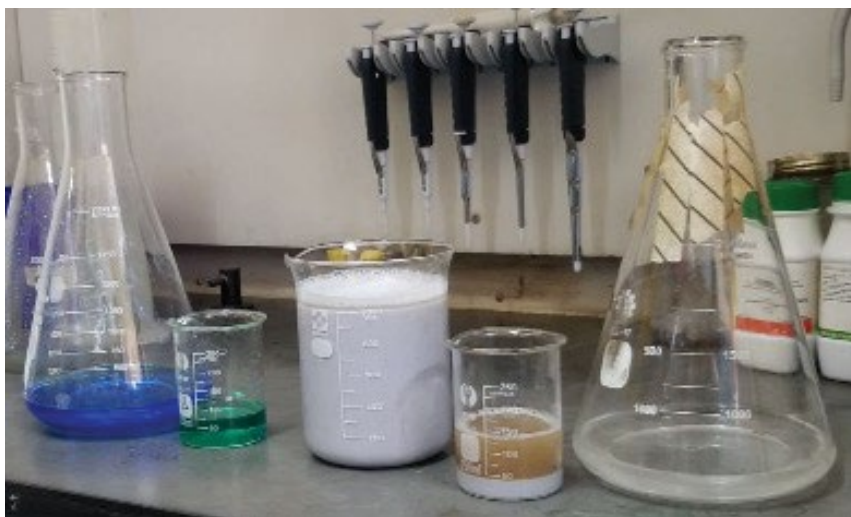
Figure 3: Erlenmeyer Flask – 250ml or larger based upon waste volume to be treated. Alternately any container can be used (food jar) but must be transparent and clean
