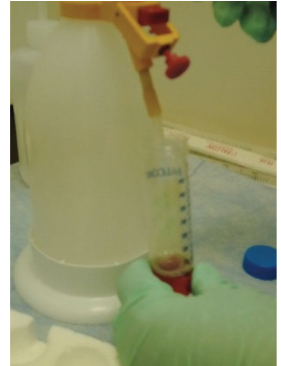
Figure 5: Titrating into a conical tube (instead of an Erlenmeyer flask)
