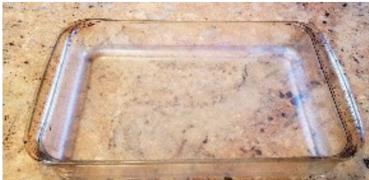
Figure 8: Shallow tray for drying precipitate. Note - do not use an aluminum pan
