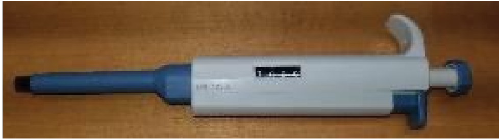
Figure 7: One pipette (0.25-5.0ml, depending on the concentration of your GTC). It can be automatic and adjustable or a traditional glass pipette. A variable pipette may be necessary.
