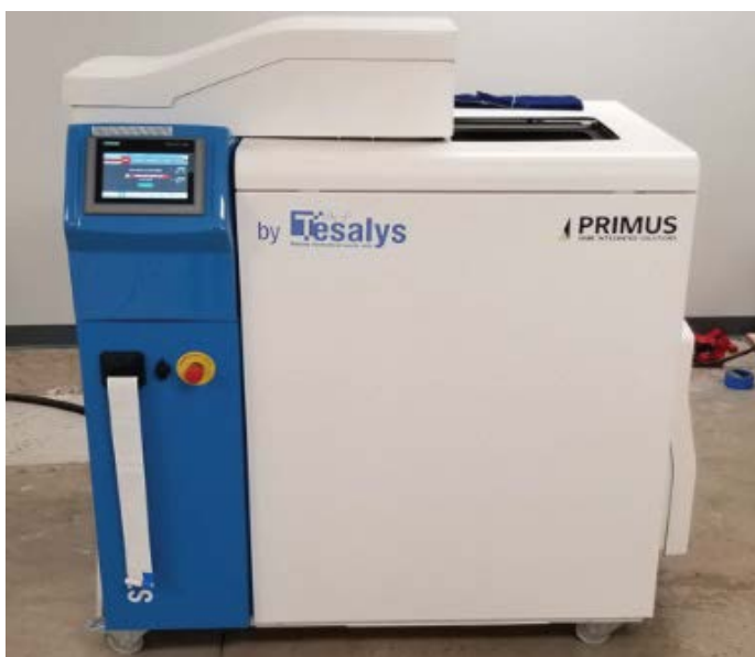
Figure 31 Tesalys autoclave (Integrated shredder)
