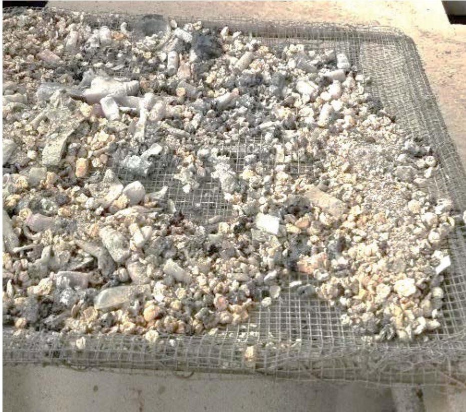
Figure 42 Bottom ash from incinerator (Note intact medication vials)
