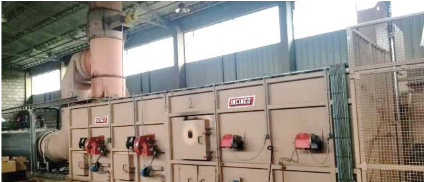
Figure 24 Fixed hearth incinerator - Incinco.
