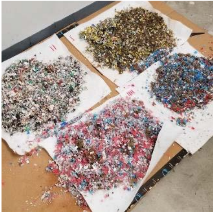
Figure 45 Tesalys autoclave processed waste
