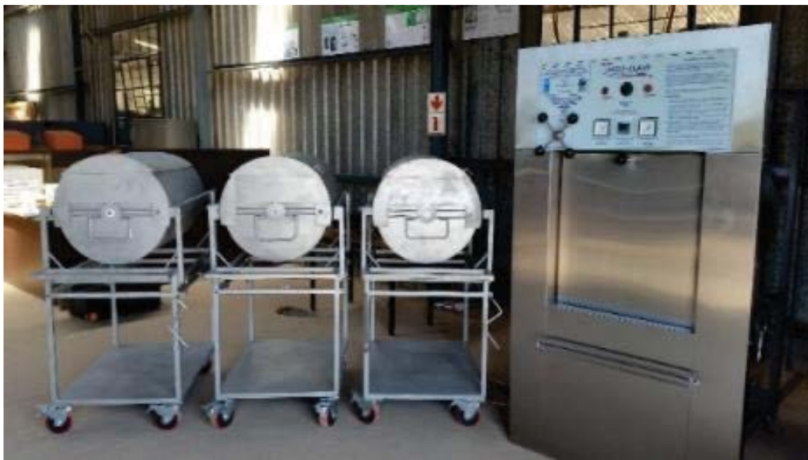
Figure 27 Medi-Clave – static autoclave – 260 liters
