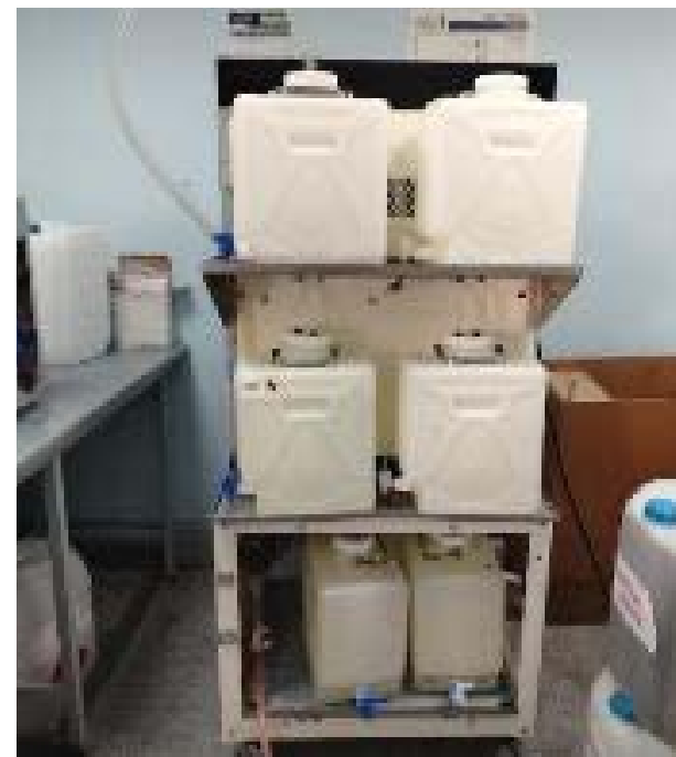
Figure 39 Solvent recovery / recycling systems CBG
