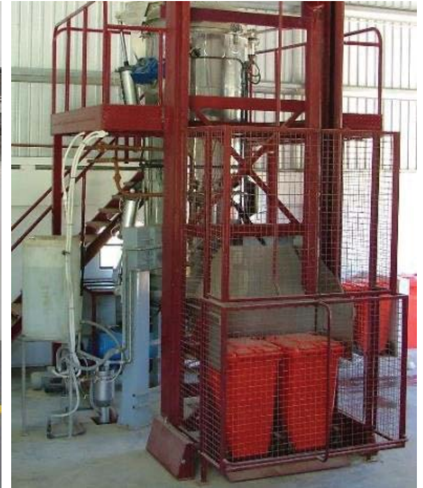
Figure 30 Ecodas hybrid autoclave (Integrated shredder)
