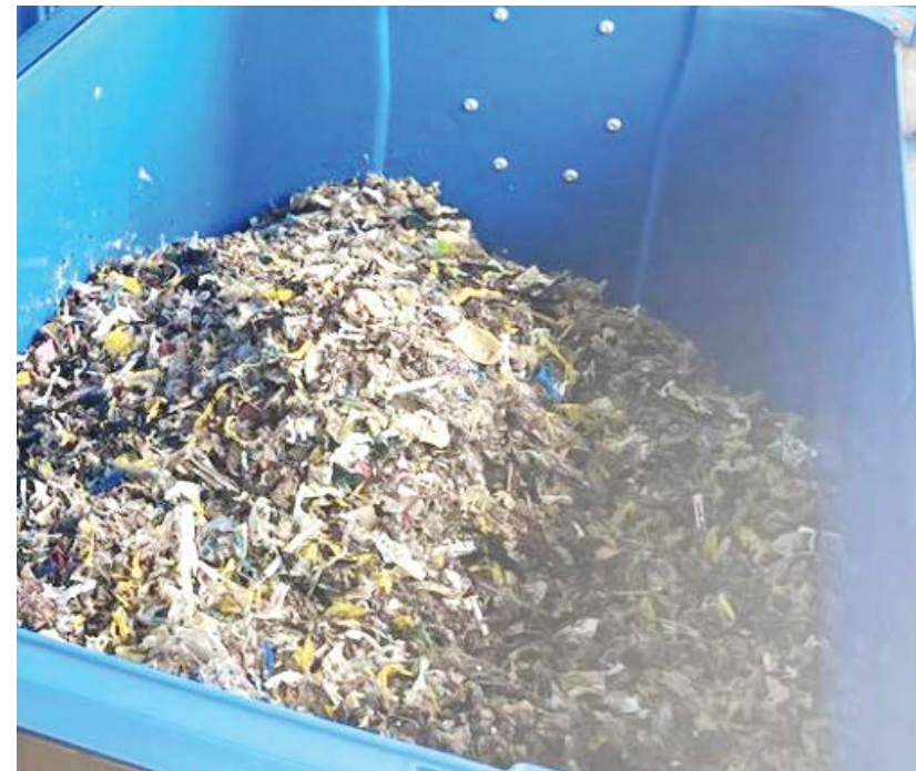
Figure 44 Ecosteryl microwave shredded waste
