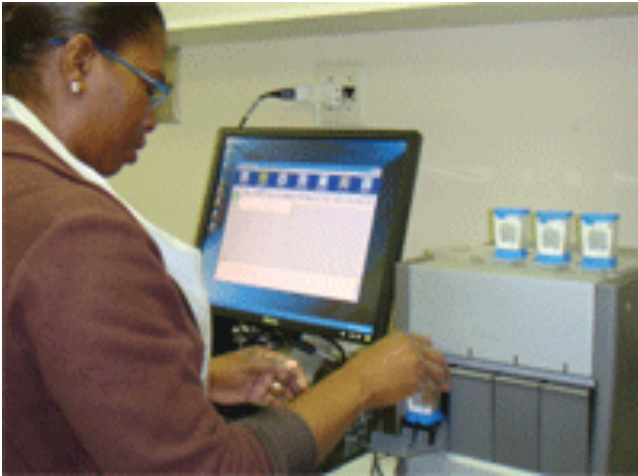
GeneXpert located at Facility interfaced with the ALIS
